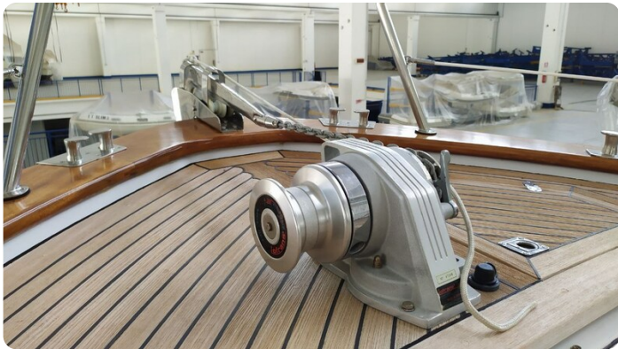
Apreamare 9 Open - Windlass Detail
