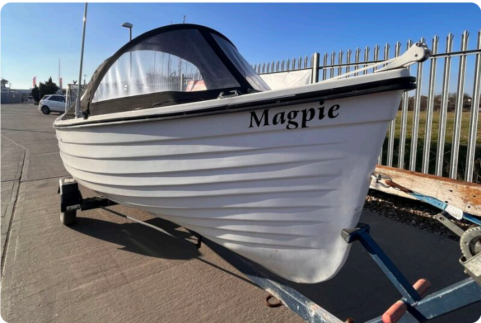
Fisherman 17 clinker boat - clinker style hull
