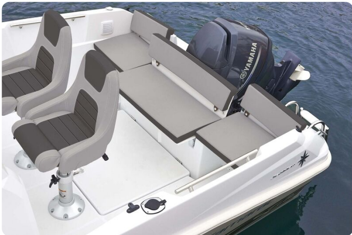
Jeanneau Cap Camarat 5.5 WA - aft sliding bench for engine to trim and tilt
