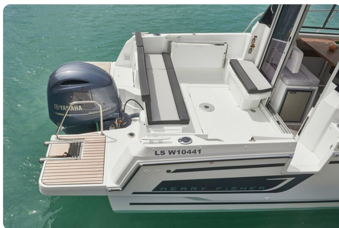
Jeanneau Merry Fisher 795 Series 2 - folding port side bench in aft cockpit
